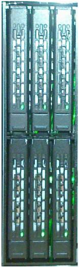
As only about 100 MB per second can be transmitted via a standard 1 GB network card, powerful DRBD clusters remain reserved for the rack computers with the ArchivistaVM. With SATA3 and SSD disks, this is no longer the case with the new models; with six disks and triple redundancy, a throughput of up to 800 MB per second can be achieved. With 10 GB network cards, the data can be transferred to another ArchivistaVM box in real time.
