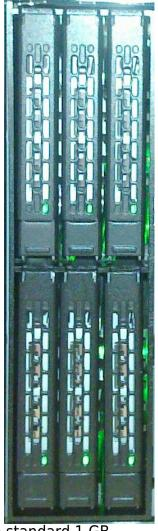
As only about 100 MB per second can be transmitted via a standard 1 GB network card, powerful DRBD clusters remain reserved for the rack computers with the ArchivistaVM. With SATA3 and SSD disks, this is no longer the case with the new models; with six disks and triple redundancy, a throughput of up to 800 MB per second can be achieved. With 10 GB network cards, the data can be transferred to another ArchivistaVM box in real time.
