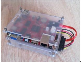
But as we all know, postponed does not mean abandoned and so it was that we ordered two Cubietruck computers for a short period of time. These are, of course, a good deal more expensive, but they incorporate more efficient hardware. Instead of the 512 MB offered by the Raspberry PI, the Cubietruck provides 2 GB (2048 MB), and a 2.5-inch hard drive can also be connected.
