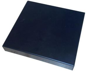
However, we struck lucky with the manufacturer of the old ArchivistaBox Dolder. For more or less the same conditions as with Cubietruck, a 64-bit hardware with 2 GB RAM is available which, based on an AMD DualCore, works very economically for a 64-bit compatible processor. When exposed to load (including hard drive), consumption lies between 8 and 12 Watts (for the entire
