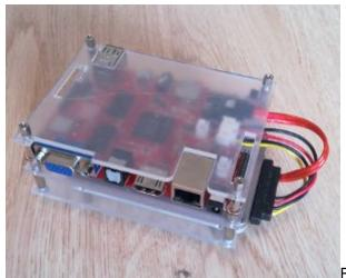
But as we all know, postponed does not mean abandoned and so it was that we ordered two Cubietruck computers for a short period of time. These are, of course, a good deal more expensive, but they incorporate more efficient hardware. Instead of the 512 MB offered by the Raspberry PI, the Cubietruck provides 2 GB (2048 MB), and a 2.5-inch hard drive can also be connected.
