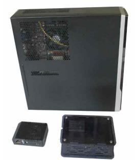
The size of the current Eiger and Matterhorn boxes (approx. 15x30x45cm) is shown in the figure below. The current size – up to the configuration level of the ArchivistaBox Säntis (approx. 3x6x9cm) – is shown bottom left and, to the right of that, the size of the other ArchivistaBox-DMS systems (approx. 5x10x15 cm).
