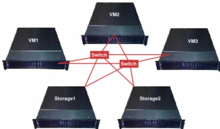
Formerly, there were four non-virtualized servers in the company, but now there are always four [virtualized] servers in the server room. However, if a server fails, then we can continue operations without interruption on the three remaining servers. Only without virtualization, we could install additional new servers as required at any time; with a cluster for virtualization, this is no longer so simple. Clusters are therefore often implemented with 3 or more VM servers.
