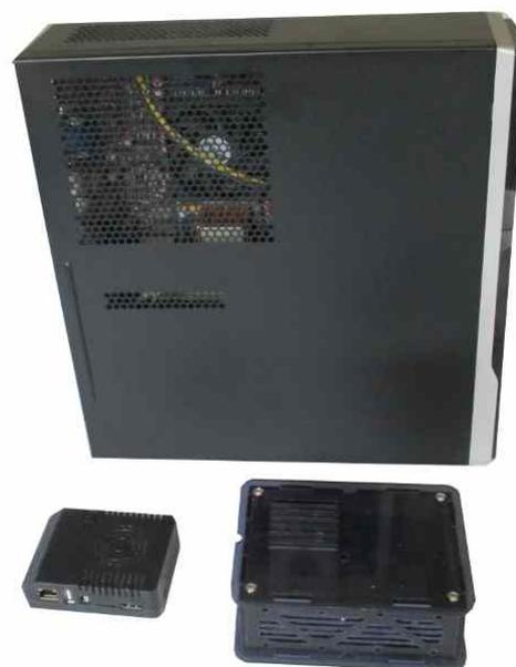
The size of the current Eiger and Matterhorn boxes (approx. 15x30x45cm) is shown in the figure below. The current size – up to the configuration level of the ArchivistaBox Sântis (approx. 3x6x9cm) – is shown bottom left and, to the right of that, the size of the other ArchivistaBox-DMS systems (approx. 5x10x15 cm).
