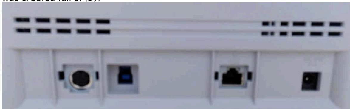
The device has USB and network connection. The device can be connected to any ArchivistaBox via USB. Unfortunately, the network connection — to put it mildly — turned out to be a loser. The IP characteristics can be set via the web interface (password is password). Unfortunately, it is not possible to specify scans in this interface, e.g. to scan to a network path.
