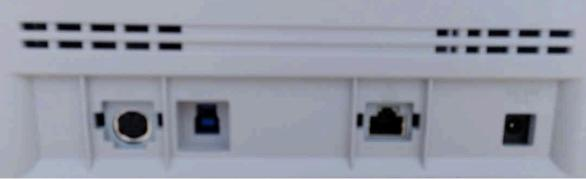
The device has USB and network connection. The device can be connected to any ArchivistaBox via USB. Unfortunately, the network connection — to put it mildly — turned out to be a loser. The IP characteristics can be set via the web interface (password is password). Unfortunately, it is not possible to specify scans in this interface, e.g. to scan to a network path.
