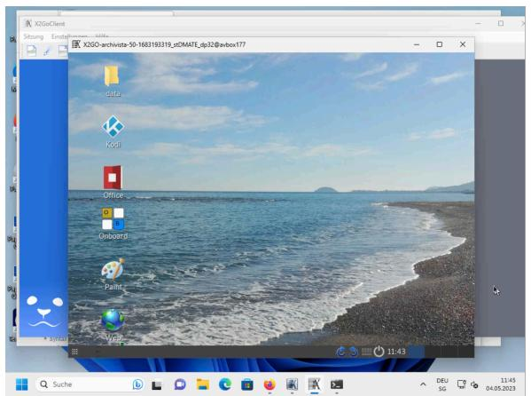
The possibilities of X2Go are almost unlimited. With the right settings (sshfs package under Linux), folders can be 'exchanged' (shared), for example. Likewise, with the package 'x2goserver-desktopsharing' it is possible to conduct remote sessions together.
