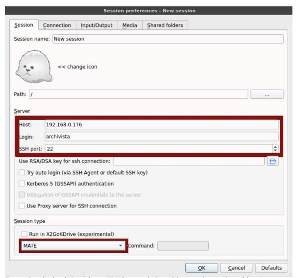
Enter the desired IP address (DNS name). Port 22 must be replaced by the address specified in the firewall for SSH access and the user must be 'archivista', as there is only this user on the ArchivistaBox or AVMultimedia. In order for remote access to work, the desktop must also be specified, whereby in our case 'Mate' is required. The process is completed with 'OK'. An entry appears in the bar on the right.
